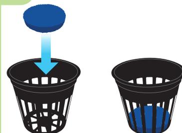
Seat blue foam pad in the base of the mesh pot
